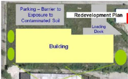
Example redevelopment plan using green infrastructure while placing barriers over contaminated soils.
